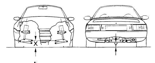
Suspension geometry should be checked only at mid-laden ride height:
